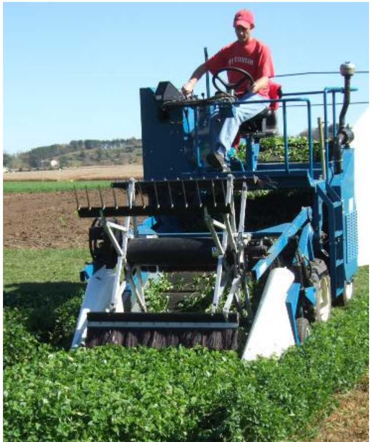
Cutting clover with special equipment that measures yield
